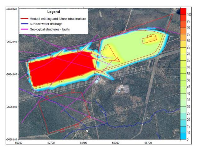
Figure 23: Model simulated pollution plumes for Scenario 1 at 50 years post closure (%) (Adapted from Groundwater Complete – 2017)
