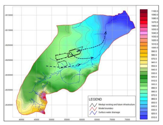
Figure 19: Groundwater Elevation Contour map (Adapted from Groundwater Complete - 2017).
